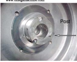
**Problem:** This post supports a sealing ring sleeve. The center of the post holds a bushing that tends to ruin the case when it fails. Getting the bushing out is difficult.
