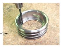
Step 2: Place the drilled sleeve back into the case with the port aligned. The drilled hole should be at the 6 o'clock position. Be sure to remove any burrs.
