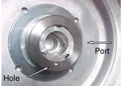
**Step 3:** Put a piece of masking tape on the drill bit to make sure the hole is deep enough to allow the pin to go all the way in.
