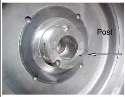
**Problem:** This post supports a sealing ring sleeve. If the sleeve comes loose, it blocks the port. The bushing in the center tends to self destruct and ruin the bushing fit in the case. This procedure addresses both of these problems.
