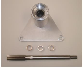
Machining of the case is necessary to install the bushing. The sleeve at the rear of the case must fit firmly on the post. Three bushings come with the tool. Omega Machine is please to announce this tool so you can repair these cases in house.
