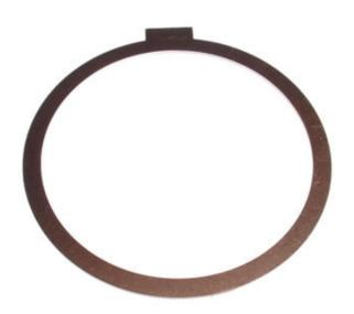
Omega Machine & Tool has come out with a steel washer/spacer to repair the 48RE rear extension housings. The snap ring wears into the case allowing the geartrain to move back and forth. This ring saves the housing by positioning the rear bearing where it belongs.
