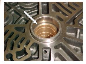
The stock bushing requires a lot of pressure to extract it. Make sure your press has good support under this Center Support or you may crack it.
