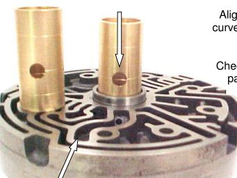
Align large hole with curved passageway as shown.
