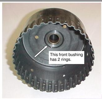
The direct drum from the 5L40E has two bushings in the support tube. On most applications both bushings are the same I.D., but different O.D. The smaller one, 98409-1 has a single identification ring on the outside of the bushing and *must* be installed first. The two ring bushing is installed last.
