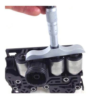
Measure and record the depth of each solenoid plunger bushing. PCA:\_\_\_\_\_ PCB:\_\_\_\_
