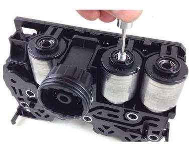
Using a 7/64 allen wrench, install the **Maxx Fluxx**<sup>TM</sup> bushings on PCA, PCB and PCC to the original depth +- 0.002-0.003
