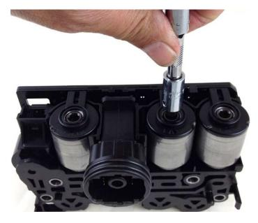
Using a T20 torxe socket remove the plunger bushing from PCA, PCB and PCC solenoid, being careful not to loose the spring between the bushing and plunger. You can use a small magnet to remove the plunger spring or use compressed air using the following procedure: Place finger forming a cup at the top of the solenoid and the with an air nozzle at an angle and gently blow air into the solenoid being careful not to loose the spring.
