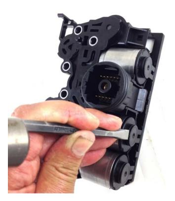
After verifying there are no electrical problems on the solenoid circuits, start by removing and discarding the caps at the end of the PCA, PCB and PCC solenoids.
