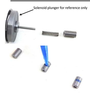
Install the plunger solenoid springs back inside the PCA, PCB and PCC solenoids. Place a drop of loctite on the center of the new Maxx Fluxx<sup>TM</sup> plunger bushing. Patent Pending.
