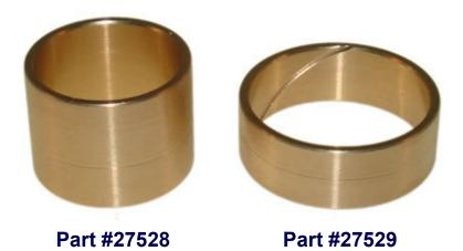
These are front and rear stator bushings for the A130/A140/A240 series Toyota transmission. The 27528 also fits the U340 front stator position. The stock replacement bushings are too sloppy and allow too much leak-by resulting in TCC slip code P0770 & P0741.
