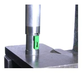
Using an arbor or hydraulic press, press on the end of the aluminum plug and watch for the stem to seat in the solenoid can. Apply just enough force on top of the crimp tool to crimp the lip of the shell over the control valve stem.
