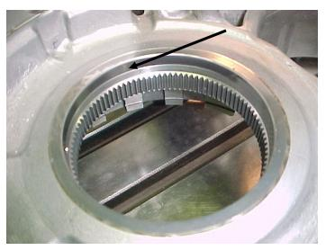
The AW 55-50SN family of transmissions comes in Maximas, Saturn Vues, Volvos, and Saabs. Transmission failure is a result of spun and worn bushings. The case wears and the transmission loses its centerline, causing bushings to fail.
