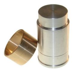
The front planet on the AX4N has a bearing in it. The bearing comes apart or has damaged the main shaft to the point you would think you need another shaft. This bushing replaces the bearing. The installed tool, part #15314 is shown in the picture and is sold separately,
