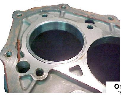
**Solution:** Omega's sleeve remounts the bearing back on it's original bore location. The sleeve has a lip or "hat" that seats in a recess to keep the snap ring from pushing it back into the case.
