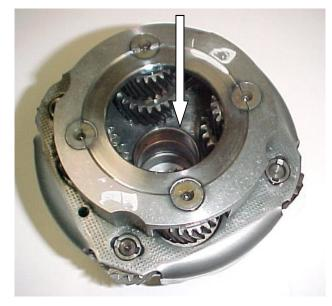
This planetary unit from a AW-5550-SN has a common flaw. The bushing closest to the sun gear is poorly supported and likes to spin in the cage.
