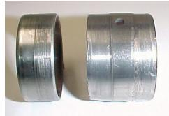
All is not lost. We bore out the cage to clean up the wear and also remove an unmachined shoulder between the bushings.
