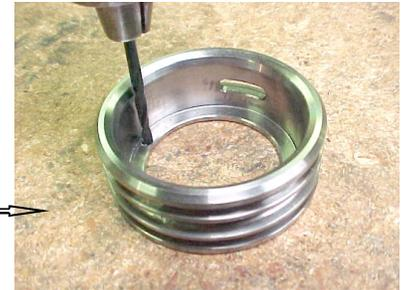
**Step 2:** Place the drilled sleeve back into the case with the port aligned. The drilled hole should be at the 6 o'clock position. Be sure to remove any burrs.
