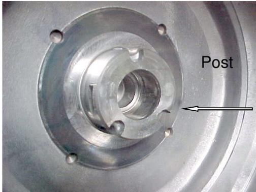
**Problem:** This post supports a sealing ring sleeve. If the sleeve comes loose, it blocks the port. The bushing in the center tends to self destruct and ruin the bushing fit in the case. This procedure addresses both of these problems.
