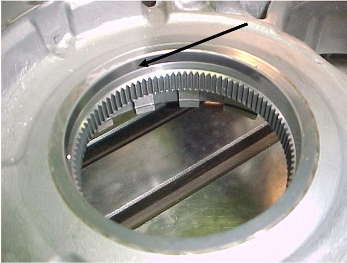
The AW 55-50SN family of transmissions comes in Maximas, Saturn Vues, Volvos, and Saabs. Transmission failure is a result of spun and worn bushings. The case wears and the transmission loses its centerline, causing bushings to fail.
