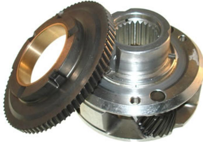
**The forward drum bushing carries a lot of load in this transmission. We've made a one piece bushing for better support. If you want just the bushing the part number is 73557. You must machine the ring gear to install the bushing.**
